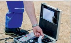
**Before starting the LWD testing** compact soil sample in a 6-inch mold to desired MC value (moisture content). Use standard compaction energy according.
